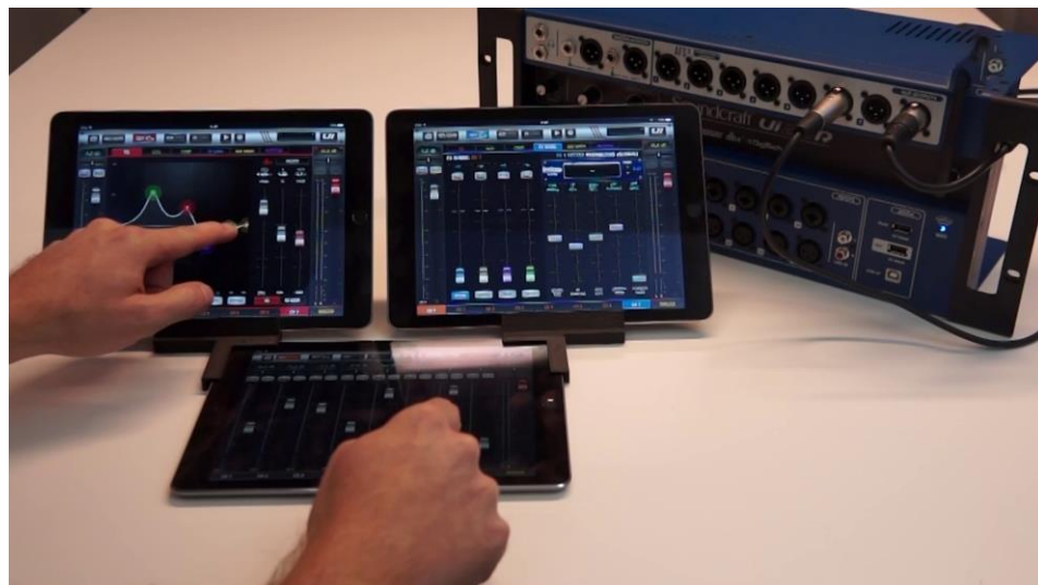
Figure 43. A user controls the commercial Soundcraft Ui24R mixing system (shown in the background and hosting the web application displayed on the tablet devices) through three tablet devices. Two 3D-printed brackets are used to create the “mixing board” layout.
