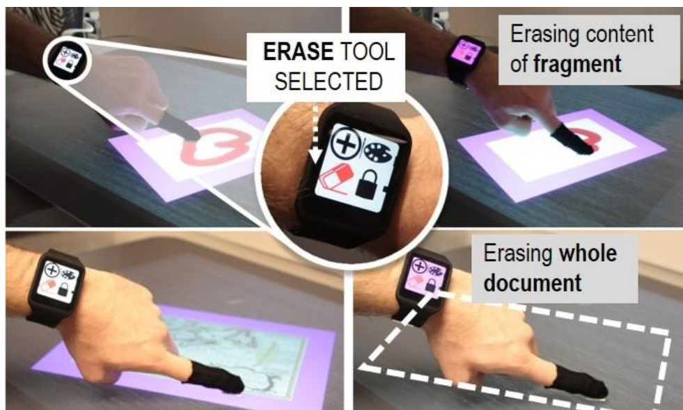
Figure 17. The erase instrument can be used to erase drawings on a canvas or image (top) and to erase documents (bottom).
