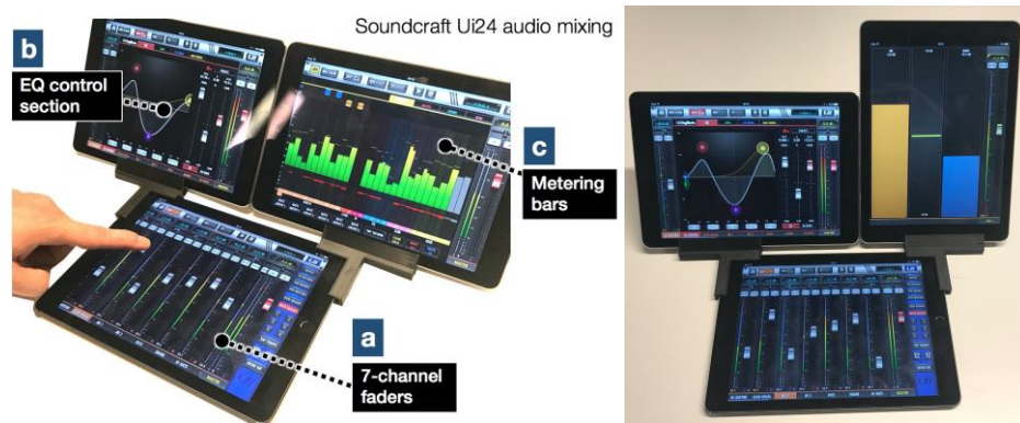
Figure 42. Audio-track mixing setup. Left: (a) control 7-channel level fader bank, (b) equaliser, and (c) metering. Right: The setup supports varying orientations of the tablets.
